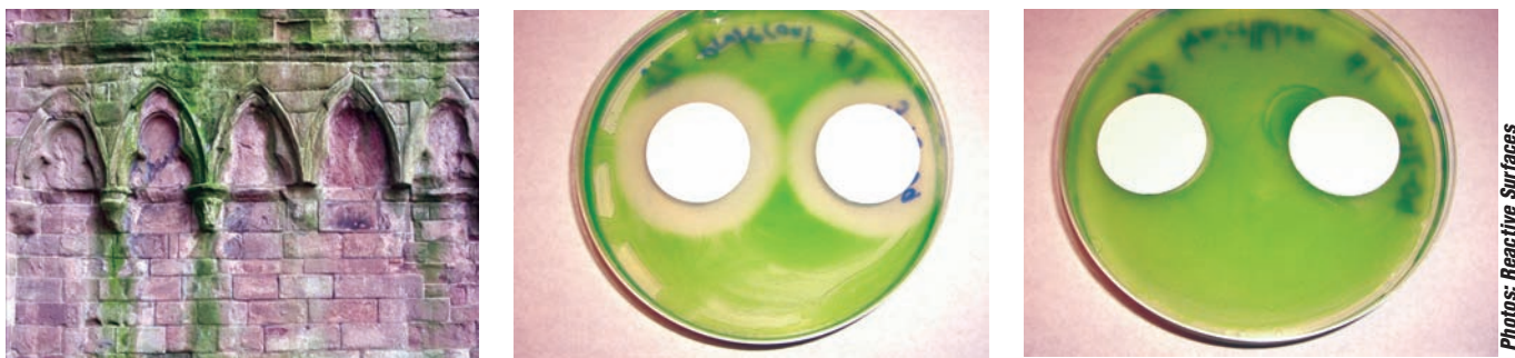
Typical algae-contaminated architectural surface (left panel) and a plate of typical algal contaminant ( Chlorella vulgaris ) showing effect of 3% ProteCoat in acrylic latex coated paper discs (middle panel) versus control lacking ProteCoat (right panel).
